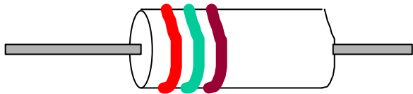
Resistor's value marked with colored bands.
