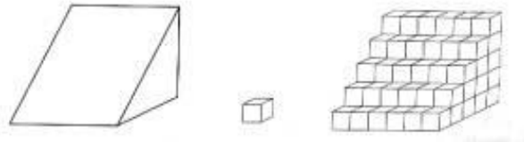
Figure 8. An object and its voxel representation (reproduced from [OCR])
