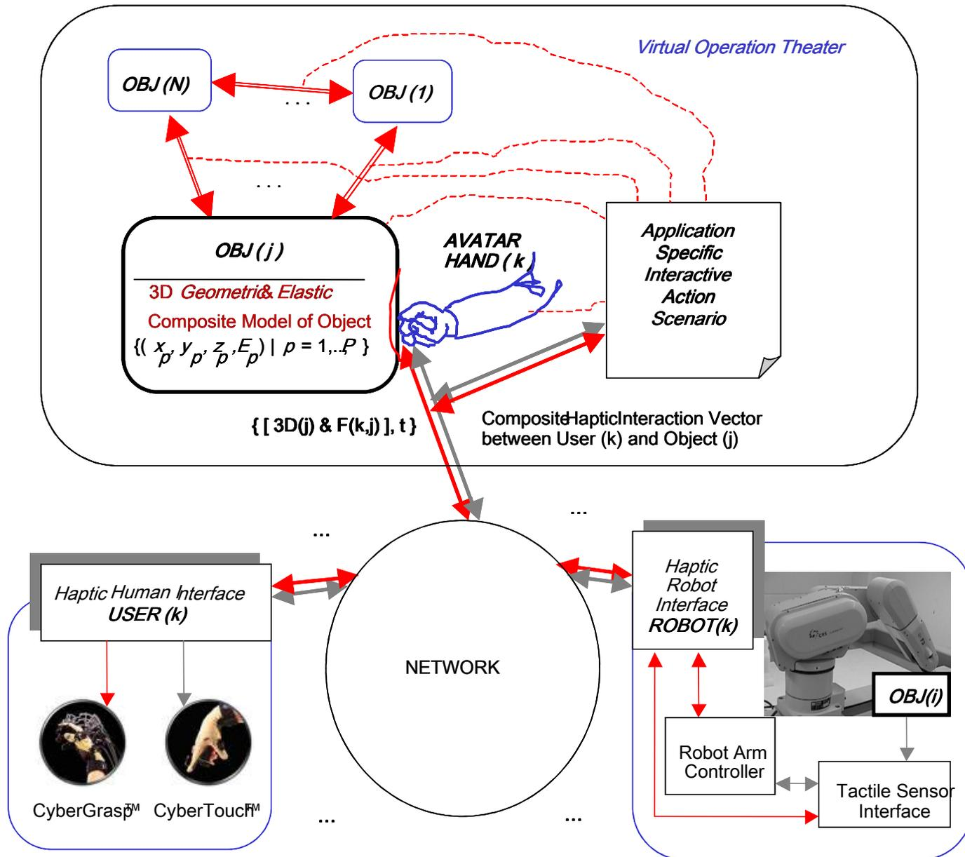
**Interactive Model-Based Hapto-Visual Teleoperation** - a human operator equipped with haptic HCI can telemanipulate physical objects with the help of a robotic equipped with haptic sensors.
