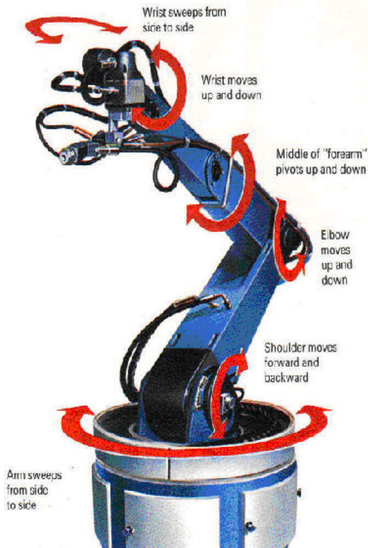
Motions of an articulated robot arm.
