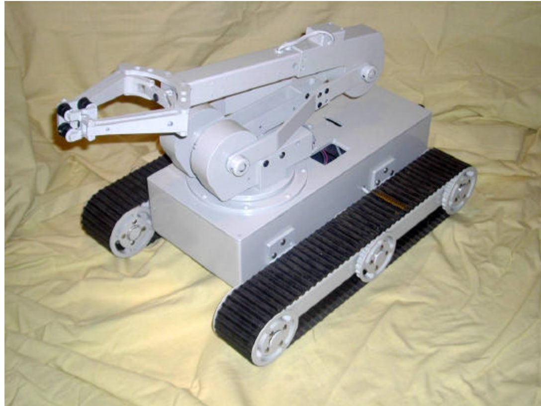
RSA platform on tracks with an onboard robotic arm for hazardous material manipulation.
