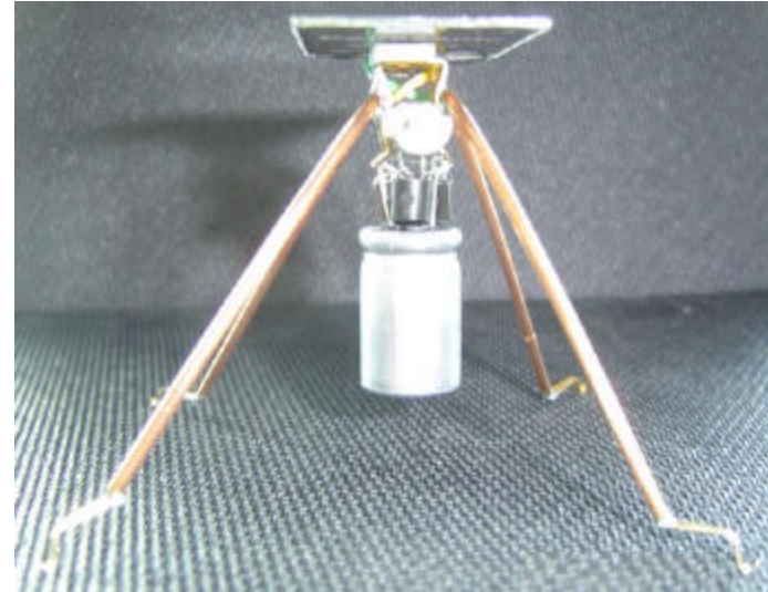
Four-leg RSA platform powered by a solar panel.
