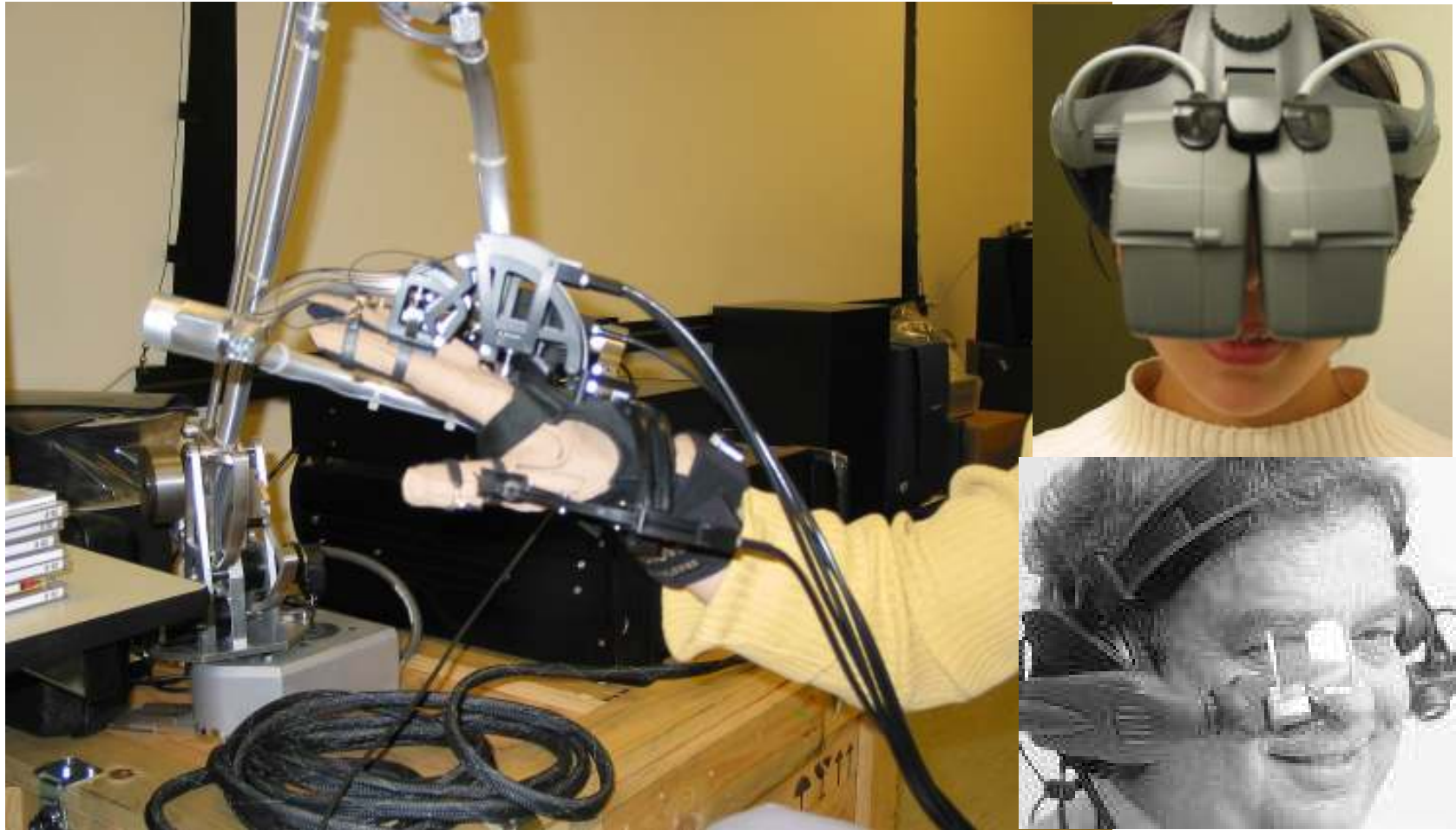
Commercial Virtual Hand Toolkit for CyberGlove/Grasp , Head Mounted Display, and see through visual display
