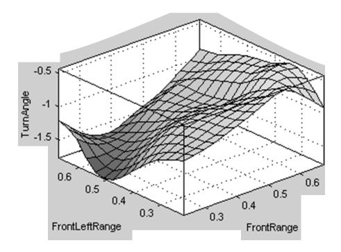
The input-output characteristics of Go-Tangent-Front-Sensor ANFIS.
