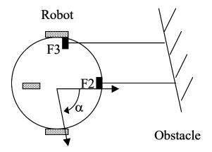
Sensors used in Go-Tangent-Front-Sensor case.
