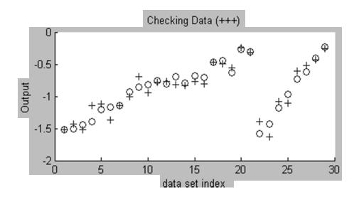
The 29 points (range, speed, turn angle)data set used for training Go-Tangent-Oblique-Sensor ANFIS. A checking data set was obtained by applying a 10% random noise to the training data set.
