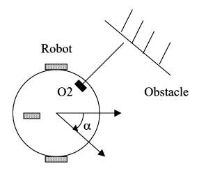
Sensors used in *Go-Tangent-Oblique-Sensor* case.
