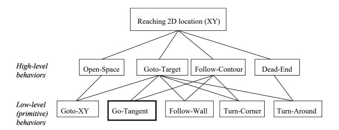
The hierarchy of the sensor-based robot behaviors
