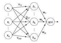
Fig. 2. The architecture of a multi-layer perceptron with a single hidden layer.
