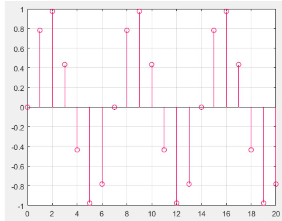
%plot() is for continuous signals and stem() is for discrete signals
