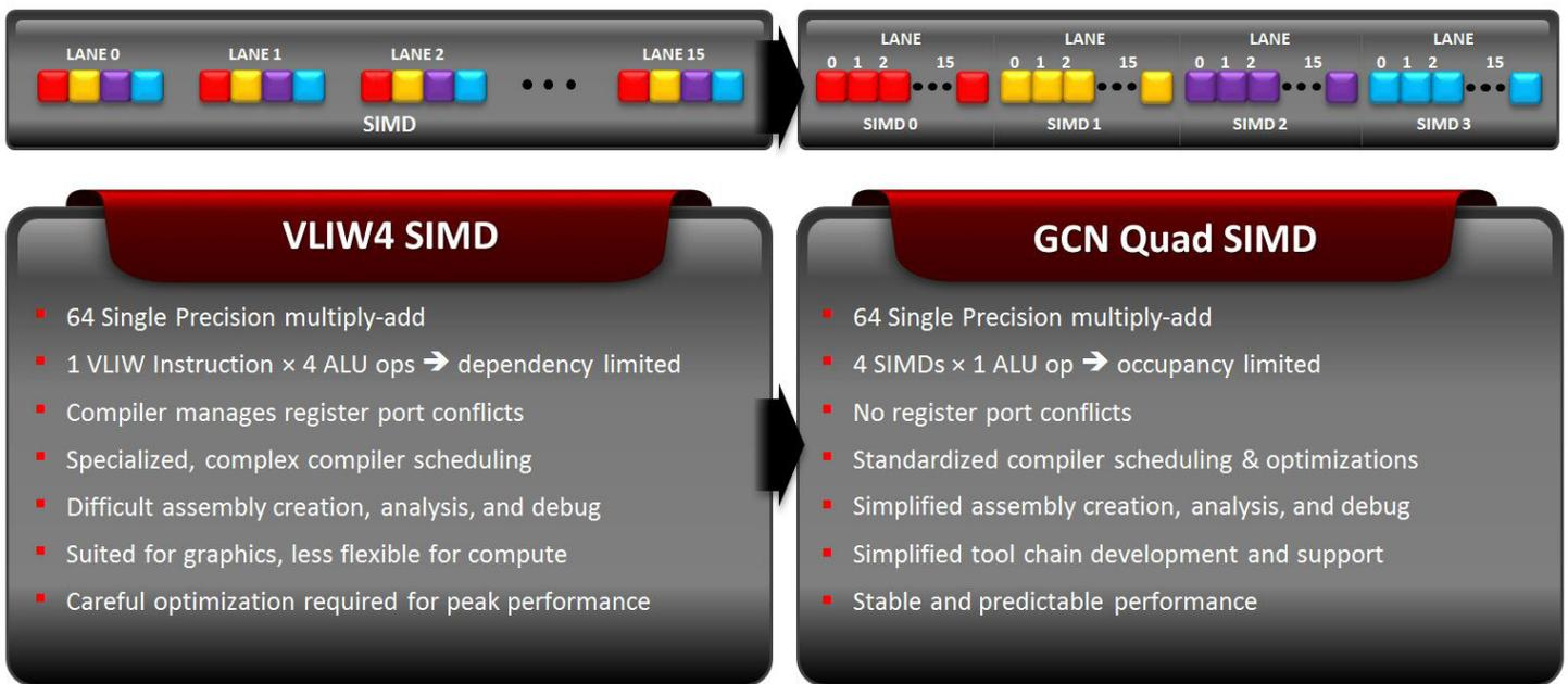
For efficiency, the SIMDs in each GCN compute unit have a combination of private and shared resources. The instruction buffering, registers and vector ALUs are private for each of the 4 SIMDs to sustain high performance and utilization. Other resources, such as the front-end, branch unit, and data cache are shared between the SIMDs to achieve area and power efficiency.
