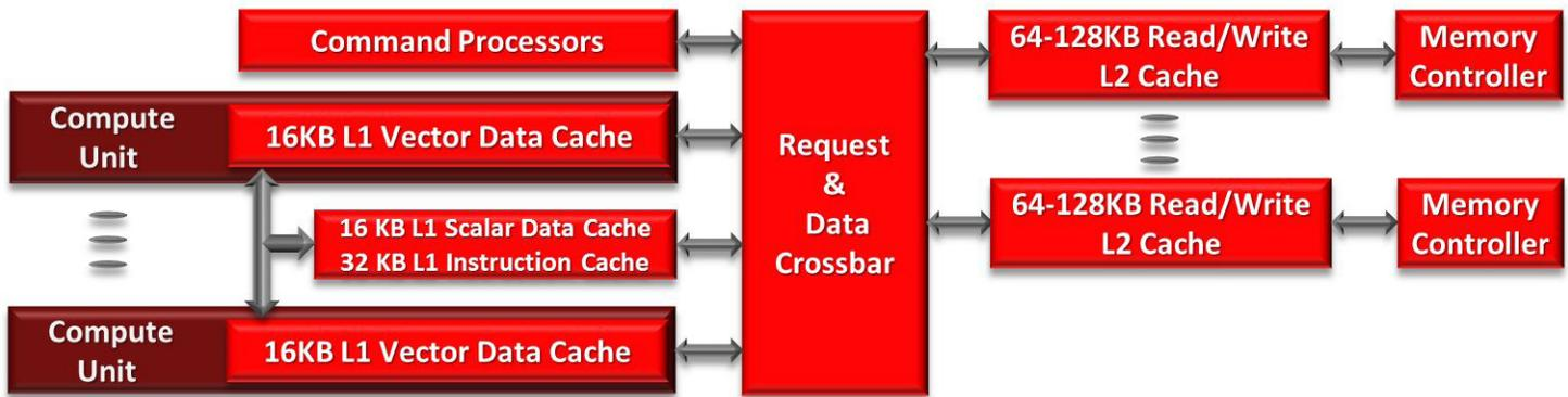
Like the L1 data cache, the L2 is virtually addressed, so no TLBs are required at all. The L2 cache is 16 way associative, with 64B cache lines and LRU replacement. It is a write-back and write allocate design, so it absorbs all the write misses from the L1 data cache. Each L2 slice is 64-128KB and can send a 64B cache line to the L1 caches.
