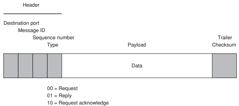
Figure E.4 An example packet format with header, payload, and checksum in the trailer.
