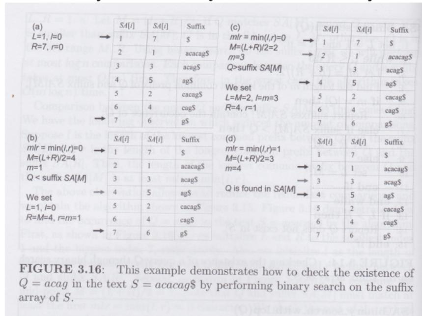
**FIGURE 3.16:** This example demonstrates how to check the existence of  $Q = acag$  in the text  $S = acacag\$$  by performing binary search on the suffix array of  $S$ .
