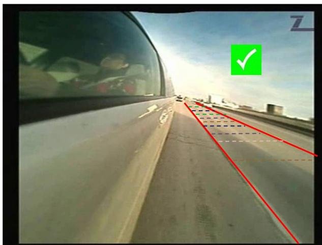
**Fig. 3.** Image decomposition into zones: The region of the image delimited by the two red lines is considered as the blindspot zone. The dashed colored lines delimit the zones considered as potentially containing a vehicle. Their sizes are estimated given the shape of the vehicle in the next lane and its distance from the camera.
