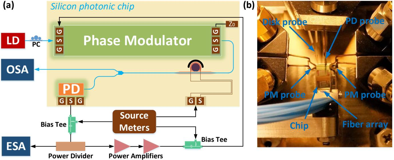
Fig. 1 (a) Schematic of the proposed integrated frequency-tunable OEO on a silicon photonic chip. LD: laser diode LD, PC: polarization controller, OSA: optical spectrum analyzer, ESA: electrical spectrum analyzer; (b) a picture of the test set-up.
