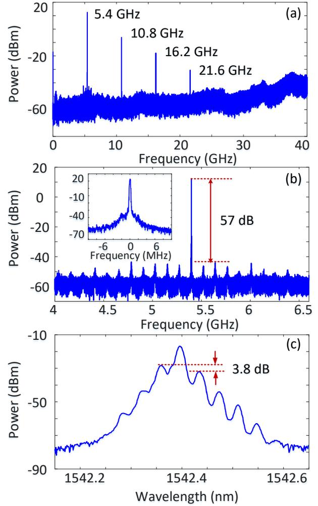
Fig. 3 (a) Electrical spectrum of the generated 5.4 GHz signal (the frequency span is 40 GHz and the resolution bandwidth (RBW) is 200 KHz); (b) electrical spectrum with a frequency span of 4 GHz and a RBW of 200 KHz. Inset shows a zoom-in view of the electrical spectrum with a frequency span of 20 MHz and a RBW of 180 KHz; (c) measured optical spectrum at the optical output grating coupler when the OEO is operating at 5.4 GHz.
