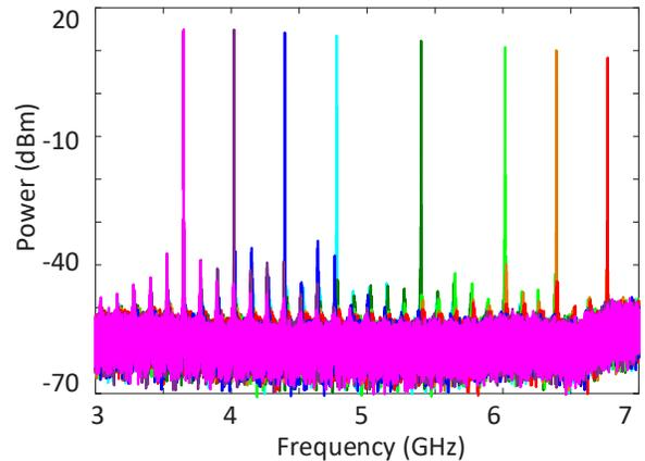
Fig. 4 Measured electrical spectrums of the generated microwave signal at different frequencies. The frequency is coarsely tuned from 3 to 7 GHz and the RBW is 200 KHz.
