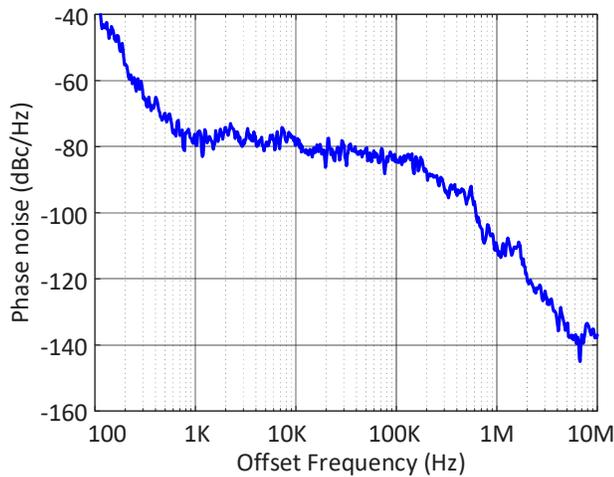
Fig. 5. Measured phase noise of the proposed OEO when the OEO is operating at 5.4 GHz.
