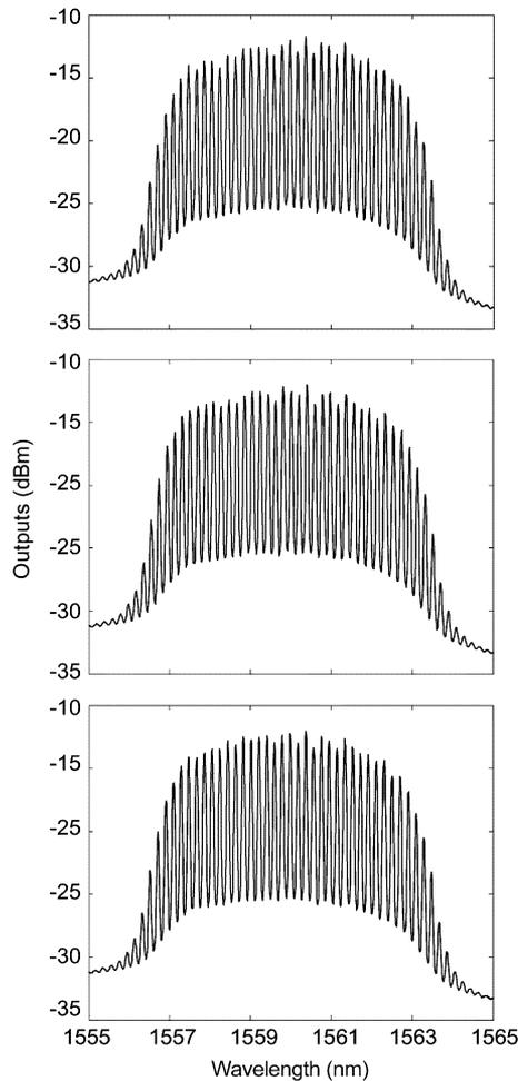
Fig. 3. Output spectra of the fiber laser taken at 10-min interval.
