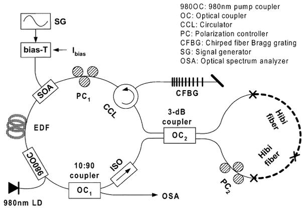
Fig. 1. Configuration of the multiwavelength EDF laser.
