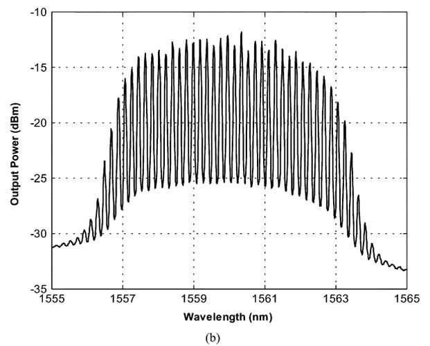
Fig. 2. Output spectrum of the fiber laser. (a) SOA biased at 86 mA without a sinusoidal modulation signal applied. (b) SOA biased at 86 mA with a 25-mV 30-kHz sinusoidal modulation signal applied.
