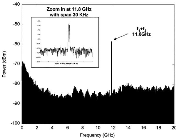
Fig. 4. Power spectrum at the output of the PD. Only the up-converted signal at 11.8 GHz is obtained and other frequency components are rejected.
