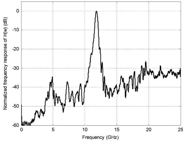
Fig. 3. Frequency response of the bandpass filter.
