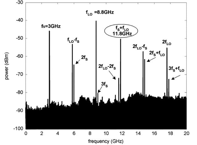
Fig. 2. Electrical spectrum of the signal at the output of the mixer, which consists of different mixing frequency components.
