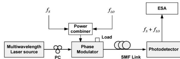
Fig. 1. Block diagram of the proposed all-optical microwave signal processor.
