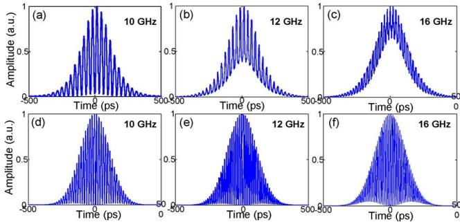
Fig. 3. Simulated output microwave pulses based on DSB modulation [(a), (b), (c)] and DSB-SC modulation [(d), (e), (f)].
