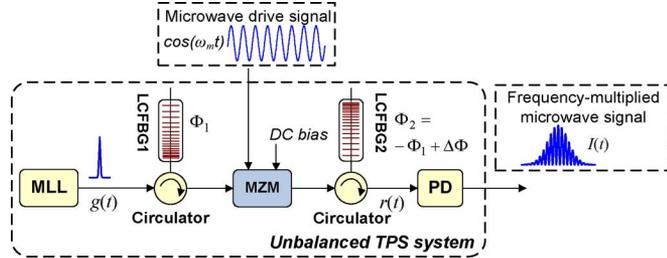
Fig. 1. Unbalanced TPS system for microwave frequency multiplication.
