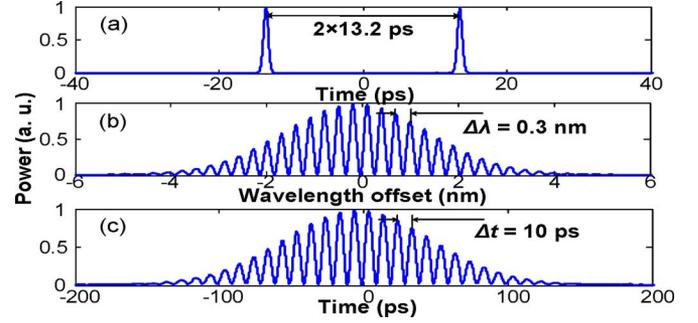
Fig. 2. Simulation results. (a) Signal at the output of the typical TPS system. (b) The optical spectrum of the signal in (a). (c) The frequency-multiplied microwave signal at the output of the entire system.
