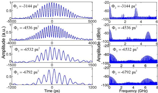
Fig. 4. Experimental results measured both in the time and frequency domains.
