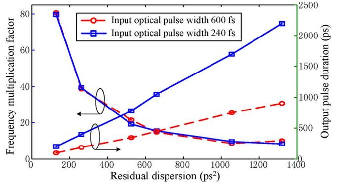
Fig. 5. Calculated frequency multiplication factor and output pulse duration as a function of the residual dispersion.
