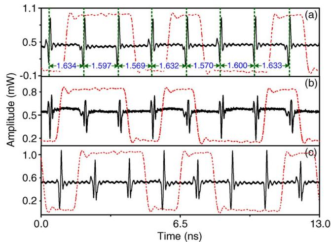
Fig. 3. Waveforms of the (a) pulse-position-modulated, (b) biphas-modulated, and (c) pulse-shape-modulated UWB signals.
