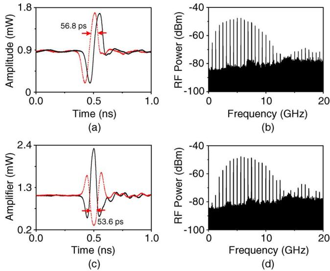
Fig. 2. Waveforms and spectra of the generated UWB pulses. (a) Generated UWB monocycle. (b) Corresponding electrical spectrum. (c) Generated UWB doublet. (d) Corresponding electrical spectrum.
