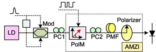
Fig. 1. Schematic of the optical UWB generator using a dual-drive intensity modulator and an asymmetric Mach–Zehnder interferometer. LD: laser diode; Mod: dual-drive Mach–Zehnder modulator; PC: polarization controller; PolM: polarization modulator; PMF: polarization-maintained fiber; and PD: photodetector.
