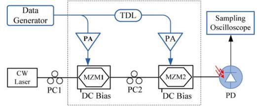
Fig. 2. Block diagram of experimental setup. The dashed lines outline the equivalent MZM. PA: power amplifier and TDL: time delay line.
