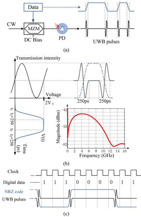
Fig. 1. Diagram showing the principle of the edge-triggered bi-phase modulation. (a) The setup of the system. (b) Generation and modulation of UWB monocycle pulses. (c) The relationship among the clock, the digital data, the NRZ code and the generated UWB pulses.
