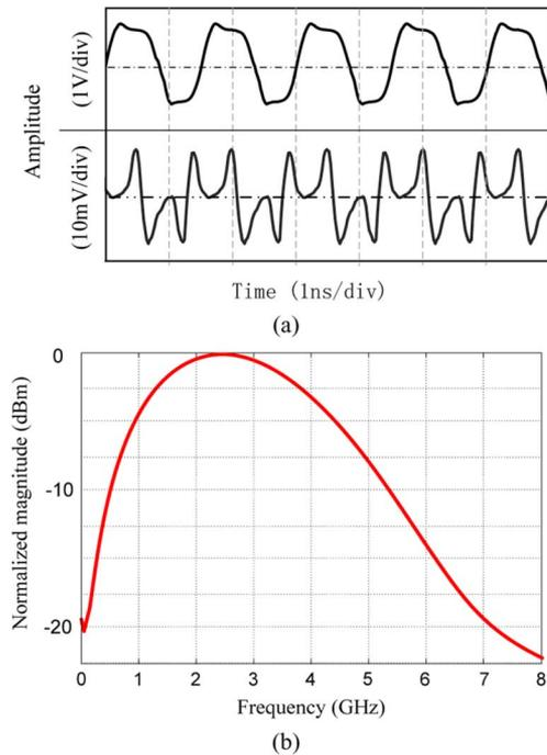
Fig. 3. The experimental results. (a) The data sequence and the generated UWB pulses. (b) The spectrum of a UWB monocycle corresponding to one rising edge of the data waveform, obtained by calculating the Fourier transform of one single monocycle taken from the experimentally generated sequence.
