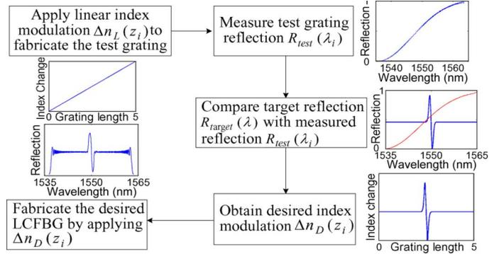
Fig. 2. Flowchart for the design and fabrication of an LCFBG with arbitrary magnitude response.
