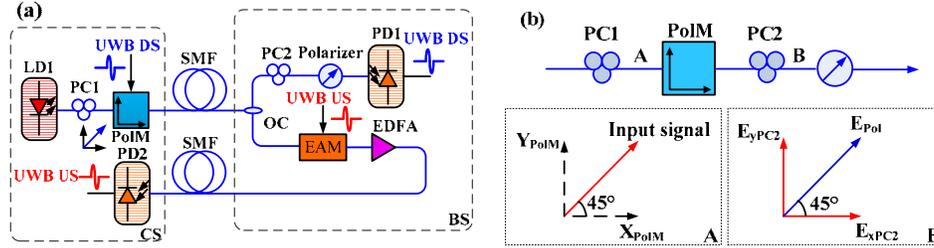
Fig. 1. (a) A bidirectional UWB optical fiber system with wavelength reuse for upstream transmission. (b) Equivalent MZM using a PolM, a PC and a polarizer.
