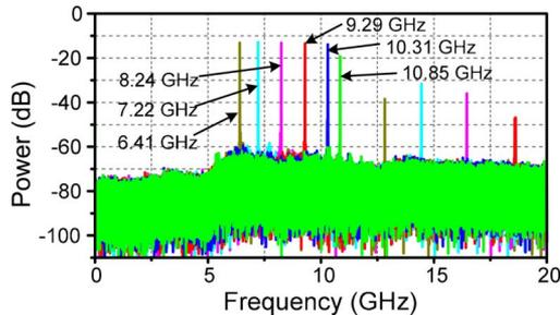
Fig. 5. (Color online) Spectra of the generated electrical signal with the frequency tuned from 6.41 to 10.85 GHz; RBW = 1 MHz.
