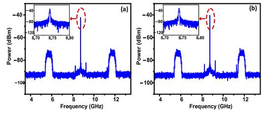
**Fig. 4.** Optical spectra for the optical signals along the (a) H and (b) V directions. Inset: Enlarged view of the generated microwave carrier.
