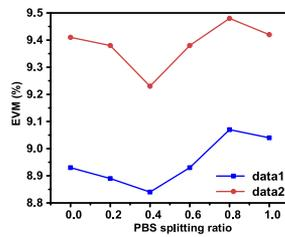
Fig. 6. Measured EVMs for different PBS splitting ratios.
