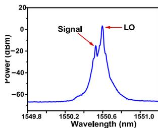
**Fig. 3.** Measured optical spectrum at the output of the OC.
