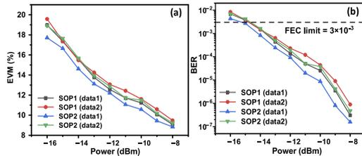
Fig. 7. Measured (a) EVMs and (b) BERs at different received optical power levels.
