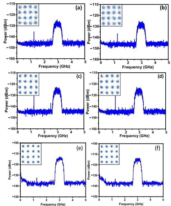
**Fig. 5.** Two downconverted and demultiplexed microwave signals along (a), (b) the H direction and (c), (d) the V direction. (e), (f) Combined signals. Inset: Constellations of the 16QAM signals.
