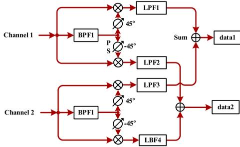
**Fig. 2.** DSP algorithm used to demultiplex the two microwave vector signals that are SOP independent.
