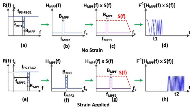
**Fig. 2.** Illustration of the operation of the interrogation system. (a) PS-FBG notch with no strain applied. (b) MPF spectral response with no strain. (c) Spectrum of the filtered signal. (d) Temporal waveform of the filtered signal. (e) PS-FBG notch with strain applied. (f) MPF spectral response with strain applied. (g) Spectrum of the filtered signal. (h) Temporal waveform of the filtered signal.
