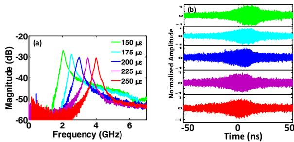
**Fig. 5.** (a) Five superimposed frequency responses of the MPF corresponding to five strains applied to the PS-FBG. (b) Corresponding five output chirped microwave waveforms with different temporal locations.
