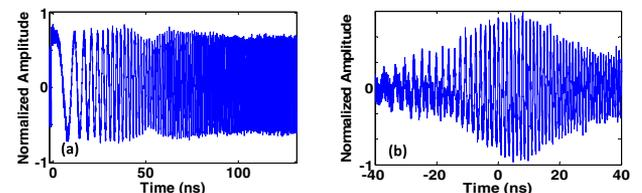
**Fig. 4.** (a) Broadband LCMW generated by an AWG. (b) Temporal waveform at the output of the MPF measured by an oscilloscope.
