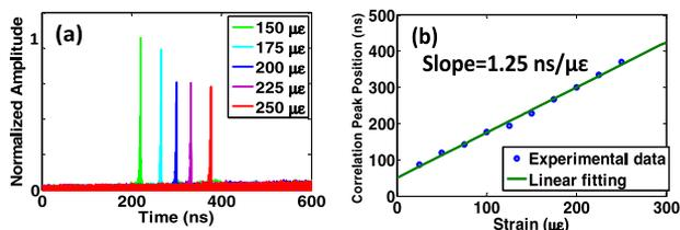
**Fig. 6.** (a) Correlation outputs of the five filtered LCMW. (b) Correlation peak position vs. applied strain. The circles are the experimental data, and the solid line shows the linear fitting of the experimental data.
