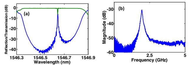
**Fig. 3.** (a) Measured reflection (green line) and transmission (blue line) spectra of the PS-FBG. (b) Measured frequency response magnitude of the MPF  $|H_{\text{MPF}}(f)|^2$  by a microwave VNA.
