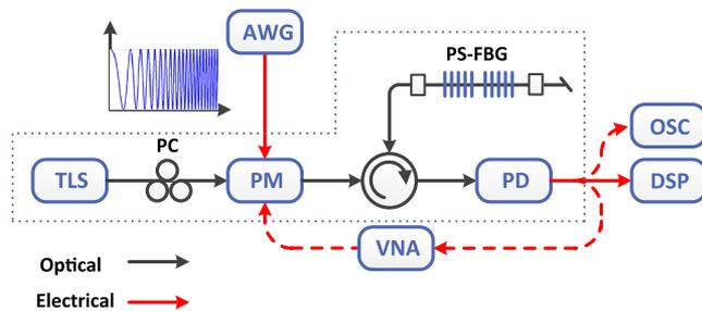
**Fig. 1.** Schematic diagram of the proposed FBG sensor. TLS, tunable laser source; AWG, arbitrary waveform generator; PM, phase modulator; PD, photodetector; VNA, vector network analyzer; OSC, oscilloscope; DSP, digital signal processor.
