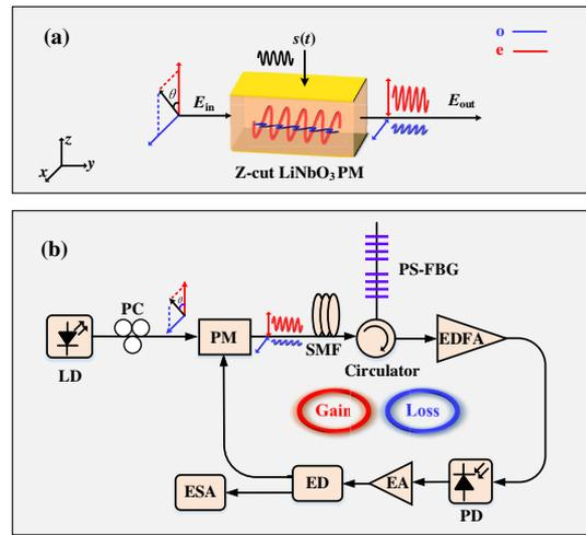
**Fig. 1.** (a) z-cut LiNbO<sub>3</sub> phase modulator that supports both ordinary and extraordinary optical modes; and (b) schematic diagram of the proposed single-loop frequency-tunable PT-symmetric OEO. LD, laser diode; PC, polarization controller; SMF, single-mode fiber; PS-FBG, phase-shifted fiber Bragg grating; EDFA, erbium-doped fiber amplifier; PD, photodetector; EA, electrical amplifier; ED, electrical divider; ESA, electrical spectrum analyzer.
