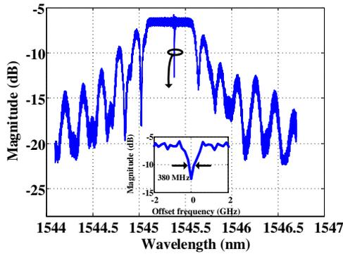
**Fig. 2.** Measured magnitude spectral response of the PS-FBG in reflection. The inset gives a zoom-in view of the notch of the PS-FBG.
