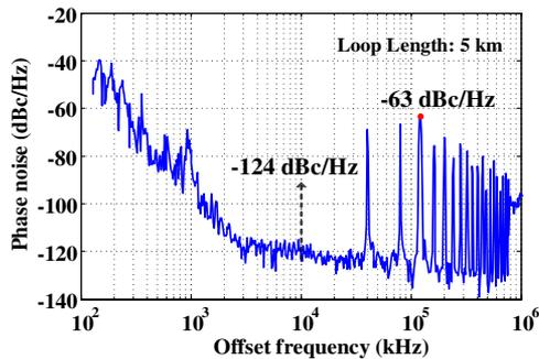
**Fig. 4.** Phase noise of the generated microwave signal at 11.8 GHz.
