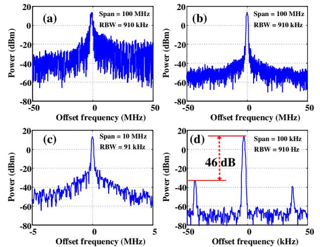
**Fig. 3.** Electrical spectra of the generated microwave signals at a central frequency of 11.8 GHz. (a) Multimode oscillation measured with a span of 100 MHz and an RBW of 910 kHz; (b) single-mode oscillation measured with a span of 100 MHz and an RBW of 910 kHz; (c) single-mode oscillation measured with a span of 10 MHz and an RBW of 91 kHz; and (d) single-mode oscillation measured with a span of 100 kHz and an RBW of 910 Hz.
