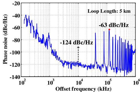
**Fig. 4.** Phase noise of the generated microwave signal at 11.8 GHz.
