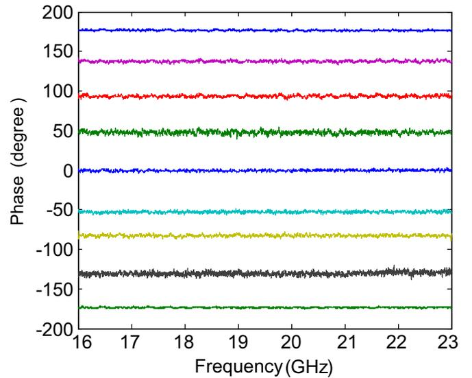
Fig. 10. Measured phase shifts at different pumping power levels. The phase shifts are independent of the microwave frequency.
