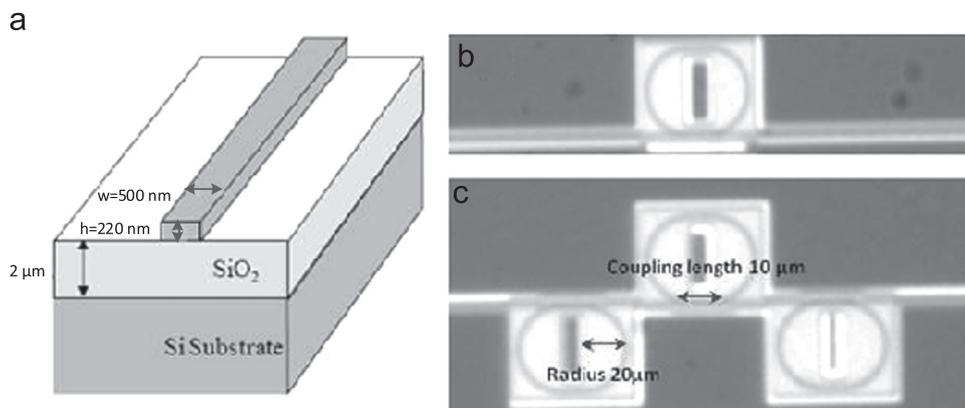
**Fig. 6.** (a) The side view of a silicon waveguide on an SOI wafer. (b) An image of the fabricated single MRR. (c) An image of the fabricated 3 cascaded MRRs.
