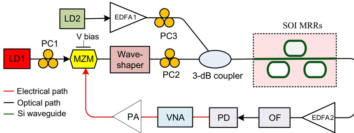
**Fig. 5.** Experimental set up. LD: laser diode, PC: polarization controller, MZM: Mach-Zehnder modulator, EDFA: erbium-doped fiber amplifier, SOI: silicon on insulator, MRR: microring resonator, OF: optical filter, PD: photodetector, VNA: vector network analyzer, PA: power amplifier.
