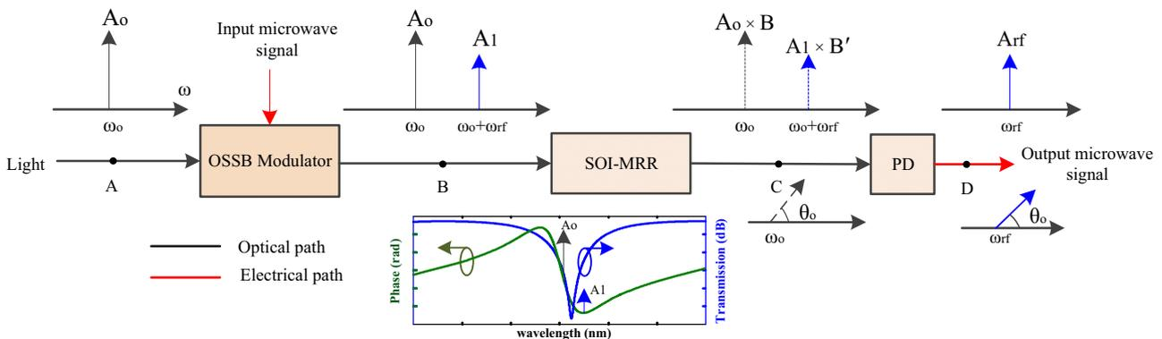
Fig. 1. Schematic of a microwave photonic phase shifter using an SOI MRR. OSSB: optical single-sideband, SOI-MRR: silicon-on-insulator microring resonator, PD: photodetector. Inset: the amplitude and phase responses of the SOI-MRR.
