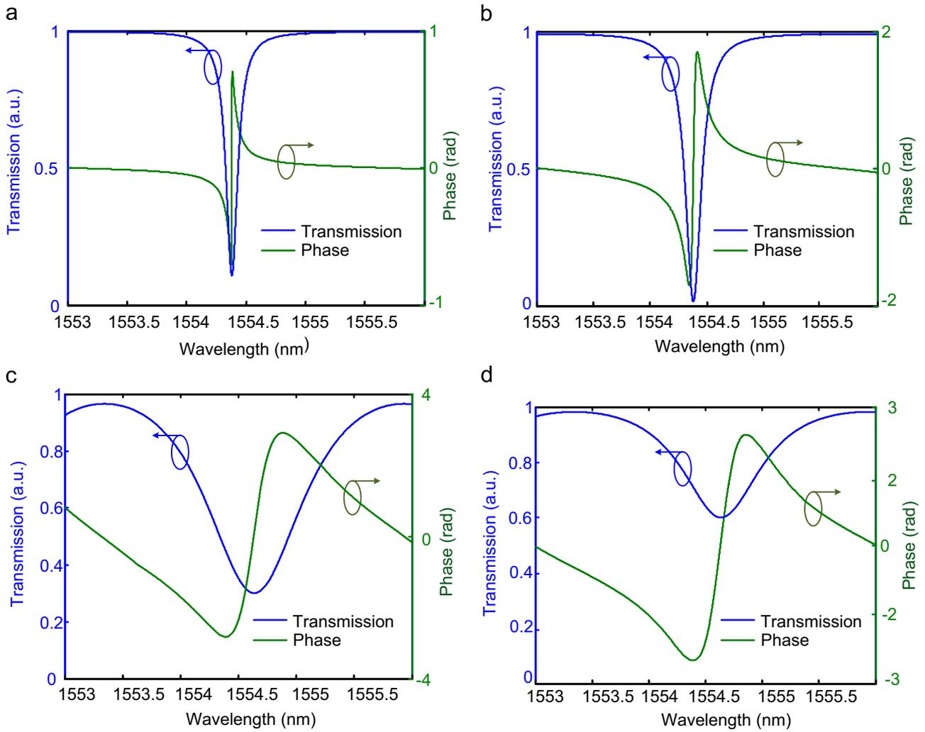
**Fig. 3.** Transmission and phase response at the through port for an MRR under different coupling conditions: (a) under-coupling with  $k=0.06$ , (b) critical-coupling with  $k^2=1-a^2=0.01$ , (c) over coupling with  $k=0.3$ , and (d) over-coupling with  $k=0.4$  ( $a\sim 0.997$ ).
