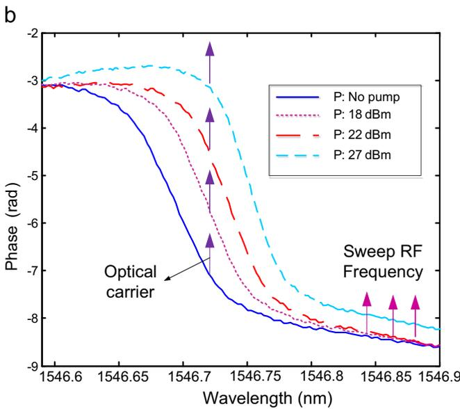
Fig. 7. (a) The magnitude response, and (b) the phase response of a single MRR showing a net redshift of the magnitude and phase with the increase of the pump power from 0 (no pump) to 27 dBm.
