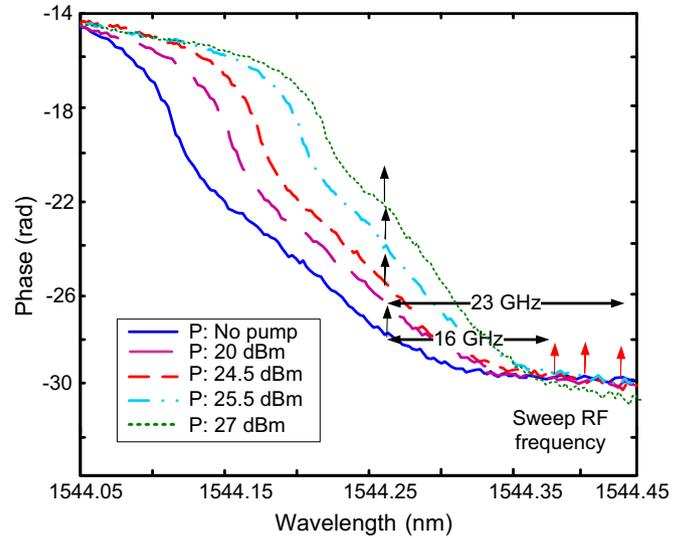
Fig. 9. The phase response of the three cascaded MRRs showing a net redshift of the phase response with the increase of the pumping power from 0 (no pump) to 27 dBm.
