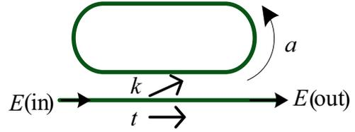
Fig. 2. The schematic of an all-pass single MRR.
