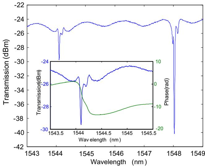
Fig. 8. Transmission spectrum of the three cascaded MRRs for the TE mode. Inset: a zoom-in view of the first notch and corresponding phase response.
