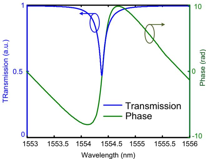
**Fig. 4.** Transmission and phase response at the through port for three cascaded MRRs under the over-coupling condition with  $k=0.4$  ( $a\sim 0.997$ ).
