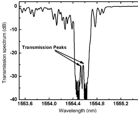
Fig. 9. Measured transmission spectrum of FBG1-3.
