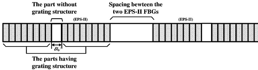
Fig. 4. Schematic diagram of FBG1-2. It consists of two cascaded EPS-II FBG's with an EPS introduced by a nonexposure part at the center of each FBG.
