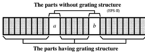
Fig. 10. Schematic diagram of FBG1-3. It consists of two EPSs (EPS-II) in a single FBG introduced by two nonexposure parts at positions *a* and *b*. The distance between *a* and *b* is 2.2 mm.
