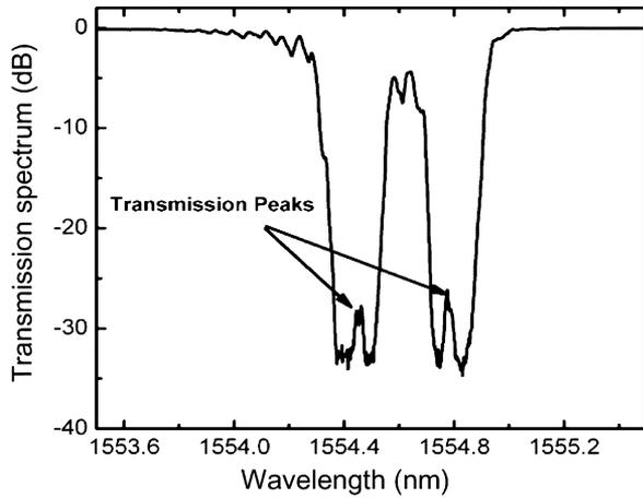
Fig. 5. Measured transmission spectrum of FBG1-2.
