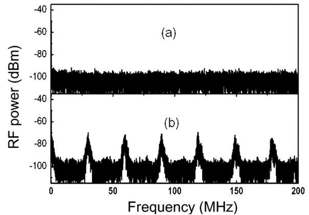
Fig. 8. Electrical spectrum of the beat signals. (a) SLM operation. (b) Multiple-longitudinal-mode operation.
