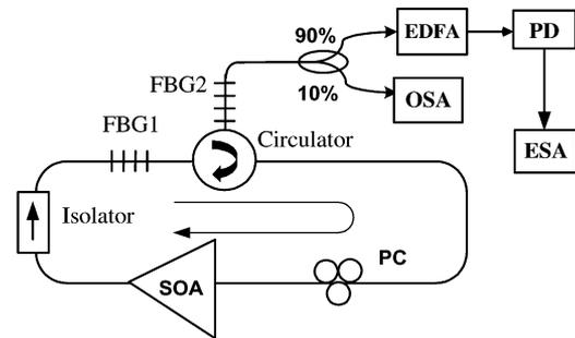
Fig. 1. Schematic diagram of the proposed dual-wavelength SLM fiber ring laser. PC: polarization controller; PD: photodetector; ESA: electrical spectrum analyzer; OSA: optical spectrum analyzer; SOA: semiconductor optical amplifier; EDFA: erbium-doped fiber amplifier.
