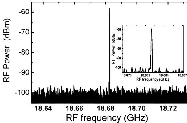
Fig. 3. Electrical spectrum of the beat signal observed at the output of the photodetector. The insert shows the detail of the RF signal with a span of 10 MHz.
