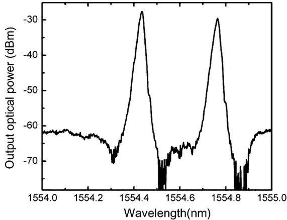
Fig. 6. Optical spectrum of the lasing output when FBG1-2 is used.
