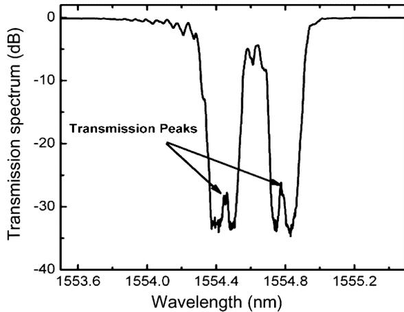
Fig. 5. Measured transmission spectrum of FBG1-2.
