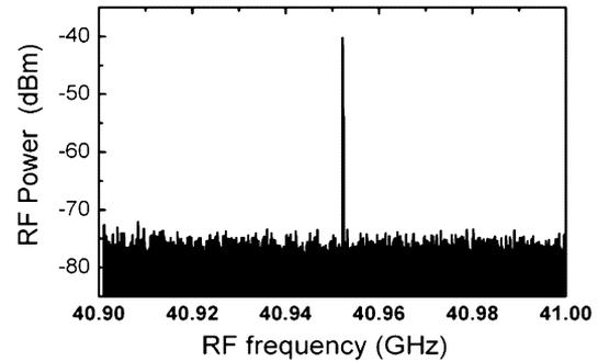
Fig. 7. Electrical spectrum of the beat signal observed at the output of the photodetector when FBG1-2 is used.
