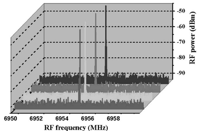
Fig. 12. Electrical spectra of the beat signal at the output of the photodetector when FBG1-3 is used. Four measurements are taken at a 15-min interval without any PC adjustment.
