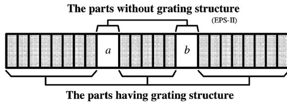
Fig. 10. Schematic diagram of FBG1-3. It consists of two EPSs (EPS-II) in a single FBG introduced by two nonexposure parts at positions *a* and *b*. The distance between *a* and *b* is 2.2 mm.
