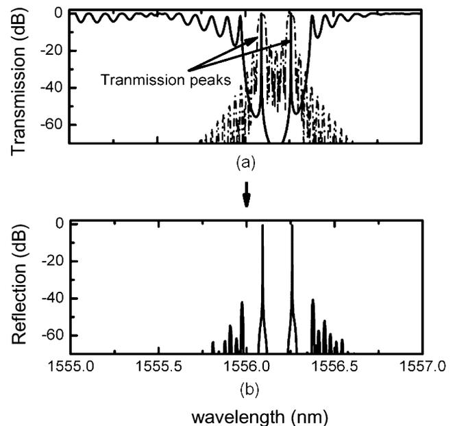
Fig. 2. Schematic optical spectra of FBG1 and FBG2. (a) Optical spectra of FBG1 (solid line) and FBG2 (dotted line). (b) The overall optical spectrum of FBG1 and FBG2 connected via an optical circulator.
