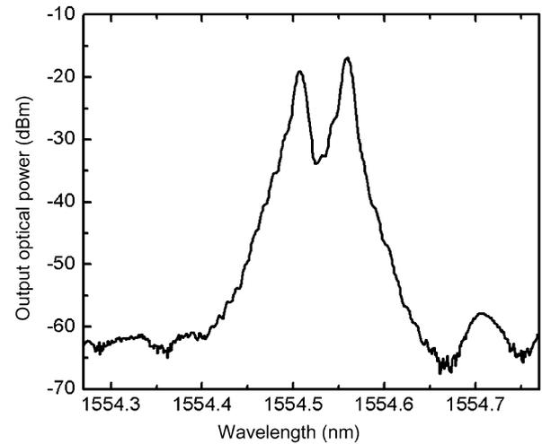
Fig. 11. Optical spectrum of the lasing output when FBG1-3 is used.
