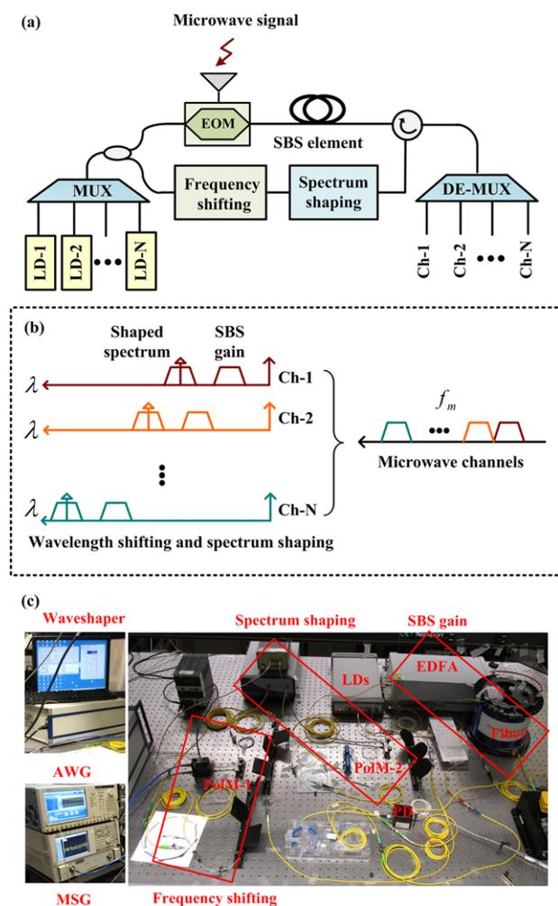
**Figure 11** Photonic-assisted microwave channelizer using a SBS processing unit: (a) schematic diagram, (b) operation principle, and (c) experimental setup. (LD: laser diode; MUX: multiplexer; EOM: electro-optic modulator; SBS: stimulated Brillouin scattering; DE-MUX: demultiplexer; Ch: channel; PoM: polarization modulator; EDFA: erbium-doped fiber amplifier; MSG: microwave signal generator; AWG: arbitrary waveform generator; PD: photodetector).
