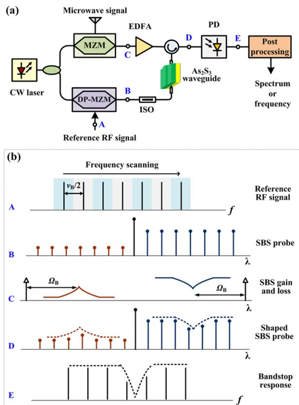
**Figure 4** Spectrum analysis system based on a scanning receiver using a chip-based photonic Brillouin filter: (a) experimental setup and (b) the optical/RF spectra measured at different points A–E [37]. (LD, laser; OC, optical coupler; MZM, Mach–Zehnder modulator; DP-MZM, dual-parallel MZM; EDFA, erbium-doped fiber amplifier; ISO, isolator; PD, photodetector;  $v_B$ , Brillouin linewidth;  $\Omega_B$ , SBS frequency shift).
