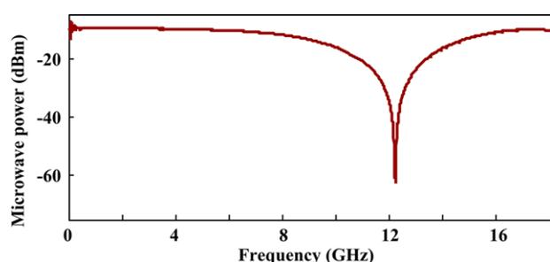
**Figure 8** Measured microwave power fading arising from chromatic dispersion.
