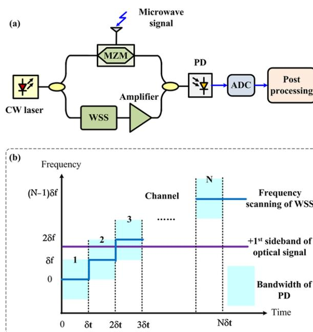
**Figure 12** Microwave channelizer based on time-division multiplexing using a wavelength-scanning source: (a) schematic diagram and (b) operation principle. (MZM: Mach–Zehnder modulator; WSS: wavelength scanning source; PD: photodetector; ADC: analog-to-digital conversion).
