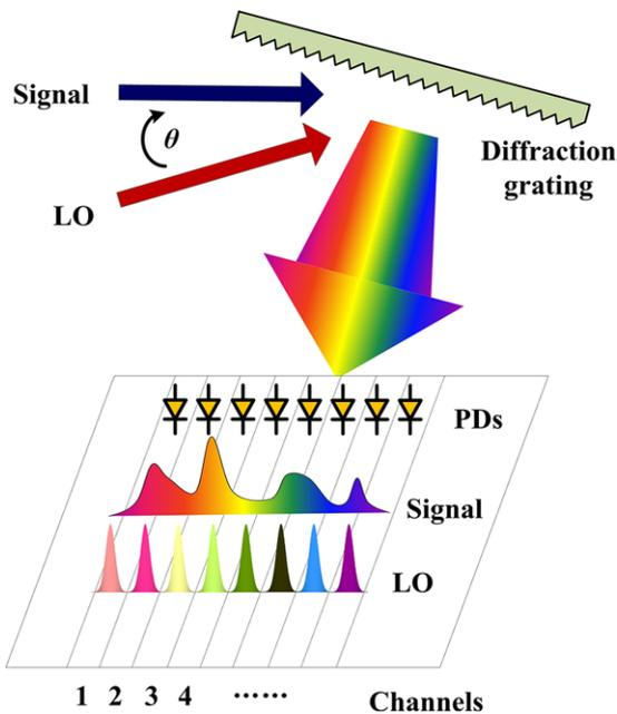
**Figure 9** Microwave channelizer based on space-division multiplexing using a free-space diffraction grating. (PD: photodetector; LO: local oscillator).
