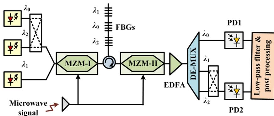
**Figure 7** Block diagram of the photonic IFM system based on an optical mixing unit with two orthogonal outputs. (MZM: Mach–Zehnder modulator; FBG: fiber Bragg grating; EDFA: erbium-doped fiber amplifier; DE-MUX: demultiplexer; PD: photodetector).
