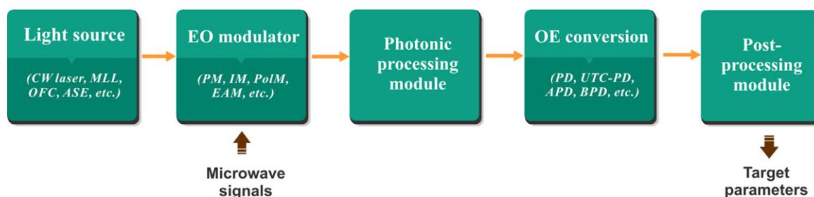
**Figure 2** Generic system architecture for photonic microwave measurements. (CW: continuous-wave; MLL: mode-locked pulsed laser; OFC: optical frequency comb; ASE: amplified spontaneous emission source; EO: electro-optic; PM: phase modulator; IM: intensity modulator; PoIM: polarization modulator; EAM: electroabsorption modulator; OE: optical-to-electrical; PD: photodetector; UTC-PD: uni-traveling-carrier photodiode; APD: avalanche photodiode; BPD: balanced photodetector).
