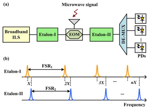
**Figure 10** (a) Microwave channelizer using a spectrally sliced incoherent source and two Fabry–Pérot etalons; (b) spectral responses of two etalons. (ILS: incoherent light source; EOM: electro-optic modulator; DE-MUX: demultiplexer; PD: photodetector; FSR: free spectral range).
