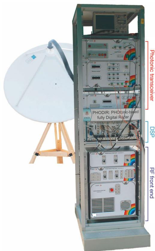
**Figure 16** Fully photonics-based coherent radar. (DSP: digital signal processing; RF: radio frequency) (reprinted from [24] with copyright permission).
