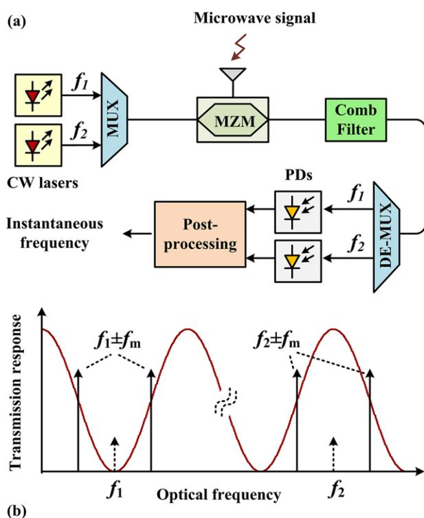
**Figure 5** (a) Schematic diagram and (b) the operation principle of a photonic IFM system based on an optical comb filter. (CW: continuous wave; MUX: multiplexer; MZM: Mach-Zehnder modulator; DE-MUX: demultiplexer; PD: photodetector).
