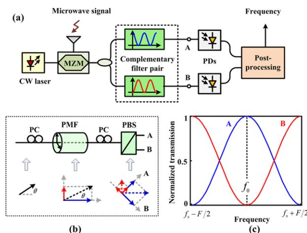
**Figure 6** Photonic IFM system based on a complementary comb filter pair: (a) schematic diagram of the system, (b) the complementary filter pair, and (c) the spectral responses of the complementary filter pair. (CW: continuous wave; MZM: Mach-Zehnder modulator; PD: photodetector; PC: polarization controller; PMF: polarization maintaining fiber; PBS: polarization beam splitter).
