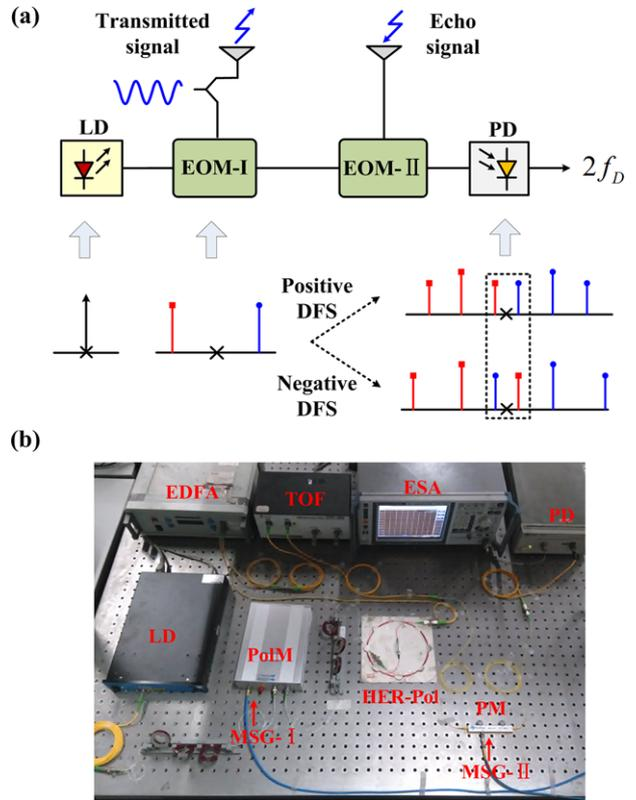
**Figure 13** Photonic DFS measurement system based on optical mixing: (a) schematic diagram and (b) experimental setup [112]. (LD: laser diode; EOM: electro-optic modulator; PD: photodetector; EDFA: erbium-doped fiber amplifier; TOF: tunable optical filter; PolM: polarization modulator; HER-Pol: high extinction ratio polarizer; MSG: microwave signal generator; PM: phase modulator; ESA: electrical spectrum analyzer).
