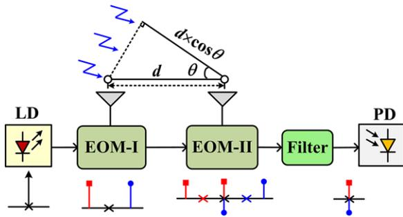
**Figure 15** Schematic diagram of a photonic AOA measurement system. (LD: laser diode; EOM: electro-optic modulator; PD: photodetector).
