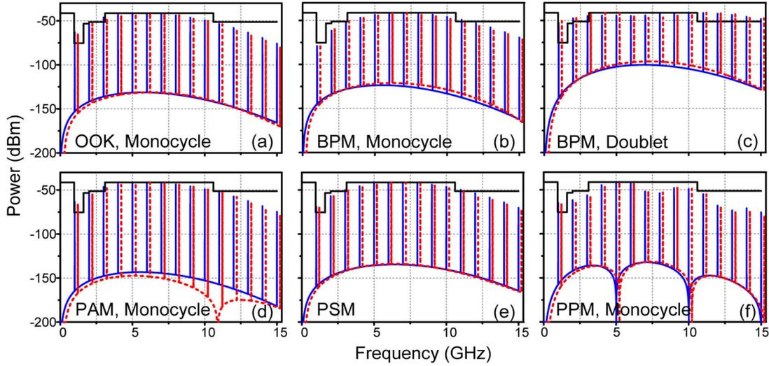
Fig. 4. PSD spectra of the radiated UWB signals with OOK, BPM, PAM, PSM, and PPM schemes. Solid lines: back to back; dashed line: with 20-km SMF transmission.  $\tau_1 = 20$  ps,  $T = 1$  ns,  $p = 0.5$ , and  $\Delta = 0$ . For OOK, BPM, PAM, PSM:  $\tau_2 = 20$  ps; for PPM:  $\tau_2 = 200$  ps.
