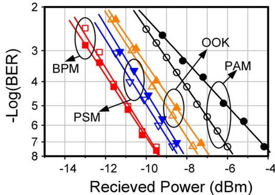
Fig. 9. BER measurements of the UWBoF system with OOK, BPM, PAM, and PSM. Hollow symbols: after wireless transmission. Solid symbols: after 20-km SMF and wireless transmission.
