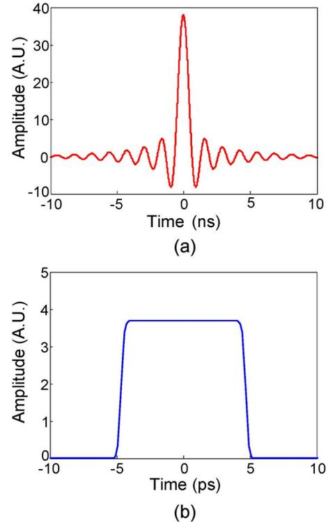
Fig. 3. Ideal case with perfect dispersion match and without SOD ( $\ddot{\Phi}=1000$  ps<sup>2</sup>,  $\ddot{\Phi}=0$ , and  $\delta\ddot{\Phi}=\delta\ddot{\Phi}=0$ ). (a) Sinc function applied to the EOM. (b) Generated square waveform.
