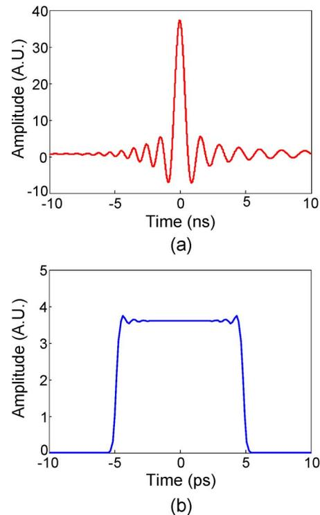
Fig. 6. Effects of the limited DAC sampling rate on the waveform generation. (a) Bandwidth-limited predistorted modulating signal. (b) Generated waveform.
