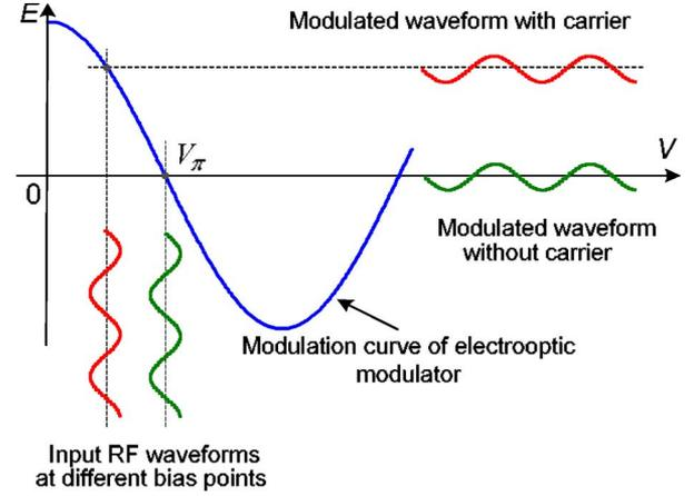
Fig. 2. Schematic diagram of the modulation process for an input RF waveform with the EOM biased at different points.
