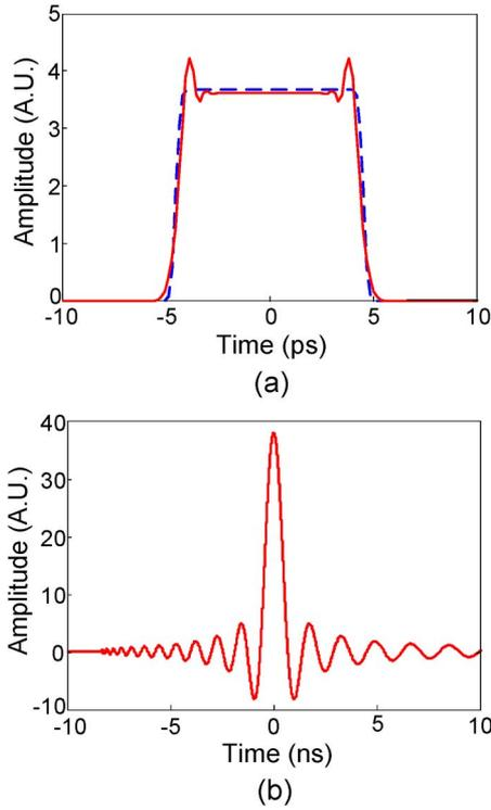
Fig. 4. Case with perfect dispersion match in FOD and SOD. (a) Generated waveform for  $\ddot{\Phi} = 1000 \text{ ps}^2$ ,  $\ddot{\Phi} = 60 \text{ ps}^3$ , and  $\delta\ddot{\Phi} = \delta\ddot{\Phi} = 0$ . Solid curve: Without predistortion. Dashed curve: With predistortion. (b) Predistorted modulating signal when  $\ddot{\Phi} = 1000 \text{ ps}^2$  and  $\ddot{\Phi} = 60 \text{ ps}^3$ .
