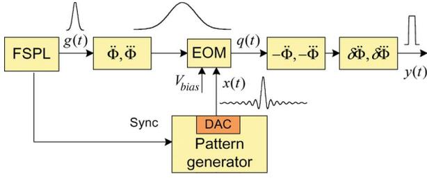
Fig. 1. Schematic diagram of the TPS system for arbitrary waveform generation (FSPL: Femtosecond pulse laser; EOM: Electrooptic modulator; DAC: Digital-to-analog converter).
