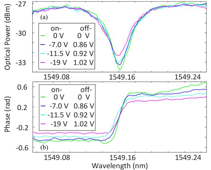
Fig. 7. (a) Tuning of the extinction ratio of the reflection notch in the +3rd channel with the notch wavelength kept unchanged, and (b) tuning of the phase jump of the reflection notch in the +3rd channel.
