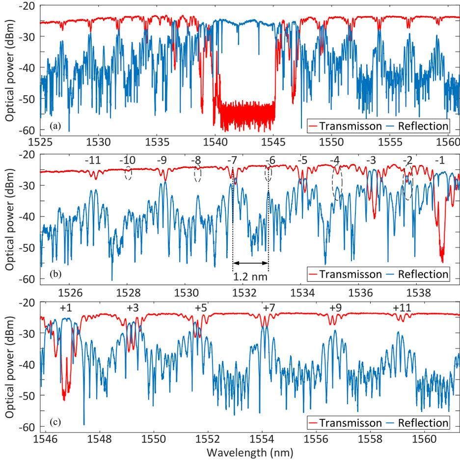
Fig. 3. (a) Measured reflection and transmission spectra of the fabricated EPS Bragg grating, (b) zoom-in view of the reflection and transmission spectra of the negative-order channels; and (c) zoom-in view of the reflection and transmission spectra of the positive-order channels.
