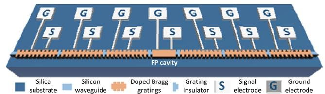
Fig. 1. Schematic view of a reconfigurable waveguide Bragg grating.
