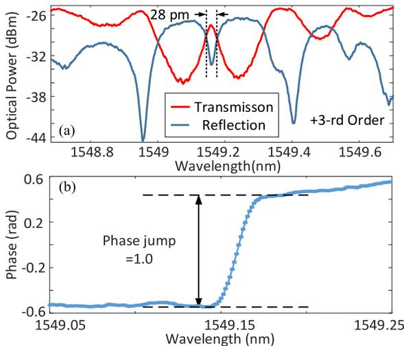
Fig. 4. (a) Measured reflection and transmission spectra of the +3rd channel and (b) the phase response of the reflection notch in the reflection spectrum.
