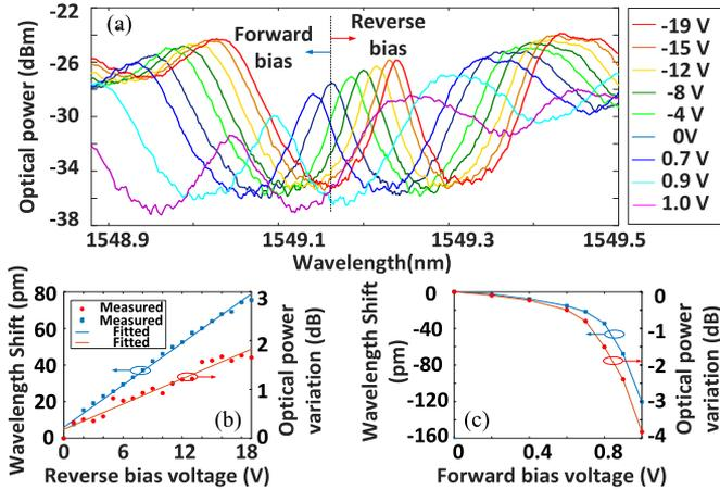
Fig. 6. (a) Measured transmission spectrum of the +3rd channel when two bias voltages are synchronously sweeping; (b) transmission window peak wavelength shifting and its power variation when the PN junctions are reverse biased; and (c) transmission window peak wavelength shifting and its power variation when the PN junctions are forward biased.
