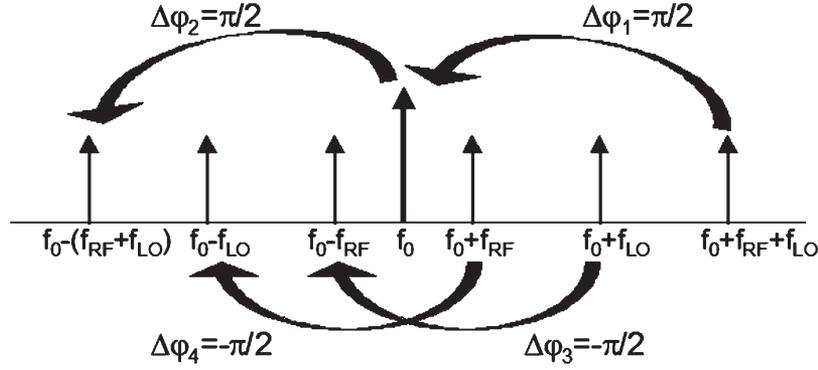
Fig. 2. Beatings of spectral lines in the optical field spectrum to generate MW mixing at  $f_{RF} + f_{LO}$ .
