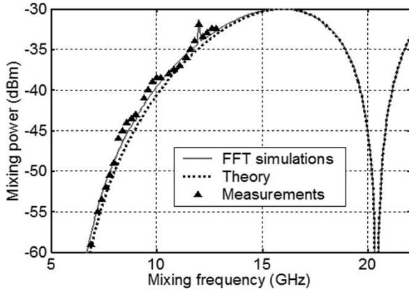
Fig. 5. Simulation/theory/measurement results of the mixing power at 10 GHz as a function of the mixing frequency.
