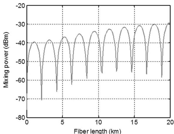
Fig. 6. FFT simulation of the mixing power at 60 GHz as a function of the fiber length.
