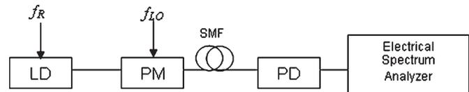
Fig. 1. Optical MW mixing system: LD, PM, SMF, and PD.
