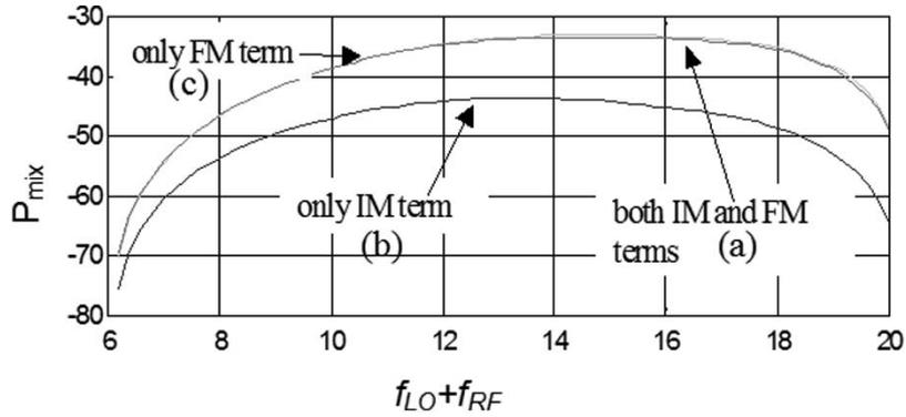
Fig. 4. Simulation of the contribution of the FM and the IM of the LD in the mixing power.
