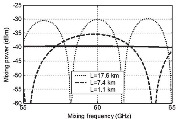
Fig. 7. FFT simulation of the mixing power as a function of the mixing frequency for three optimal fiber lengths.
