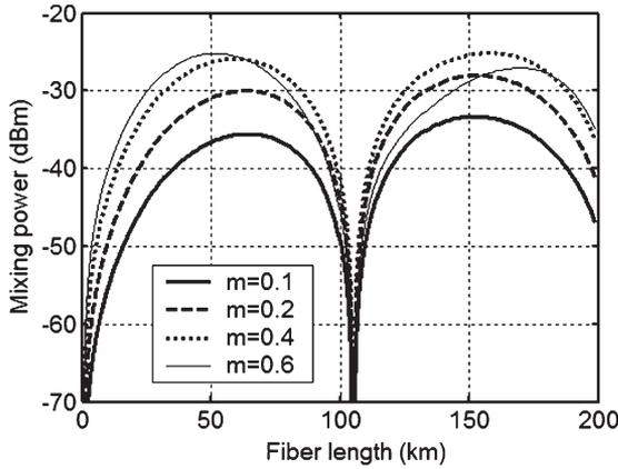
Fig. 3. FFT simulations of mixing power at 10 GHz as a function of fiber length for different IM index  $m$ .
