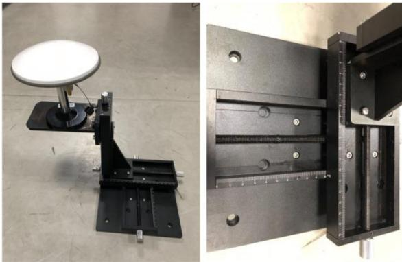
Fig. 9. The three-dimensional high precision device alignment stage used to emulate the building vibration.
