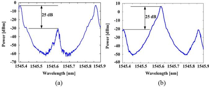
Fig. 5. Spectrums of the optical signals at the outputs of the two ports of PBS1.
