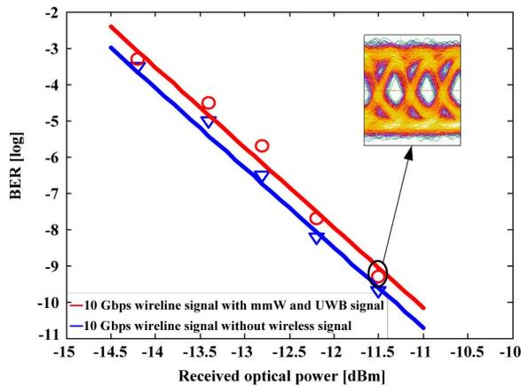
Fig. 9. BER for the transmission of a 10-Gbps wireline signal with or without simultaneous transmission of a broadband mmW and a UWB signal. Inset: eye-diagram of the 10-Gbps baseband signal with simultaneous transmission of a 1.25-Gbps mmW and a 1.25-Gbps IR-UWB signals.
