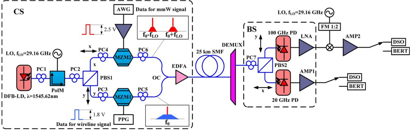
Fig. 3. Experimental setup. PPG: pulse pattern generator, AWG: arbitrary waveform generator, EDFA: erbium-doped fiber amplifier, PD: photodetector, AMP: electrical amplifier, LNA: low noise amplifier, FM: frequency multiplier, DSO: digital storage oscilloscope, BERT: bit error tester.
