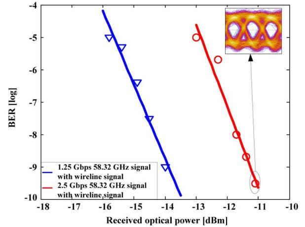
Fig. 7. BER for the transmission of a 58.32-GHz mmW signal with simultaneous transmission of a 10-Gbps wireline signal. Inset: eyediagram of the down-converted 2.5-Gbps OOK-modulated 58.32-GHz mmW signal.
