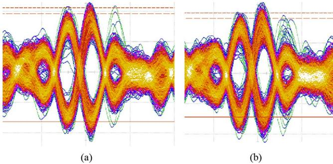
Fig. 14. Eyediagrams of the received IR-UWB signal. (a) The IR-UWB signal without simultaneous transmission of an mmW signal and a wireline signal. (b) The IR-UWB signal with simultaneous transmission of an mmW signal and a wireline signal.
