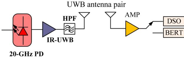
Fig. 12. Wireless transmission of an IR-UWB signal via a UWB antenna pair.
