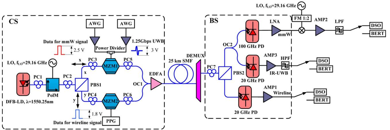
Fig. 8. Experimental setup for the simultaneous transmission of a broadband mmW, an IR-UWB and a wireline signal.
