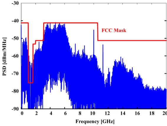
Fig. 13. PSD of the IR-UWB signal at the output of the high-pass filter.
