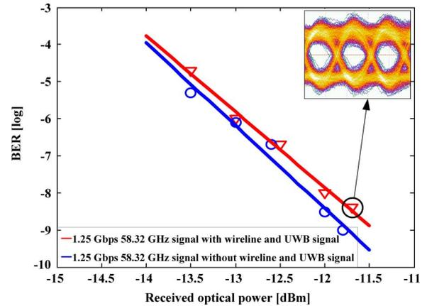
Fig. 10. BER for the transmission of a 1.25-Gbps 58.32-GHz mmW signal with or without simultaneous transmission of a 10-Gbps wireline signal and a 1.25-Gbps IR-UWB signal. Inset: eye-diagram of the down-converted 1.25-Gbps 58.32 mmW with simultaneous transmission of a 10-Gbps wireline signal and a 1.25-Gbps IR-UWB signal.
