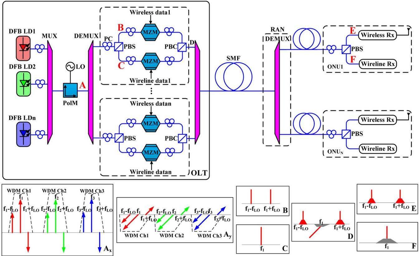
Fig. 1. Principle of the proposed hybrid broadband wireless and wireline signal over WDM-PON. OLT: optical line terminal, DFB LD: distributed feedback laser diode, MZM: Mach-Zehnder modulator, PBS: polarization beam splitter, PBC: polarization beam coupler, PC: polarization controller, MUX: WDM multiplexer, DEMUX: WDM de-multiplexer, RAN: remote access node, PBS: polarization beam splitter, Rx: receiver.
