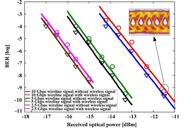
Fig. 6. BER for the transmission of a wireline signal with or without simultaneous transmission of a wireless mmW signal. Inset: eyediagram of the 10-Gbps baseband signal with simultaneous transmission of a 2.5-Gbps wireless mmW signal.
