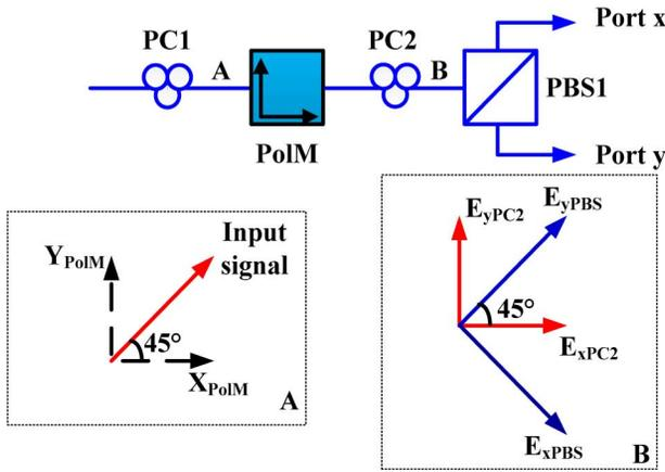
Fig. 4. Equivalent MZM using a PolM, a PC (PC1) and a PBS (PBS1).
