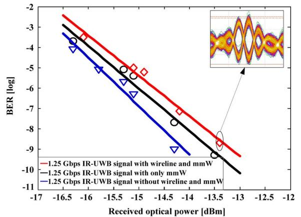
Fig. 11. BER for transmission of a 1.25-Gbps IR-UWB signal with or without simultaneous transmission of a 10-Gbps wireline signal and 1.25-Gbps 58.32-GHz mmW signal. Inset: eye-diagram of the 1.25-Gbps IR-UWB signal.
