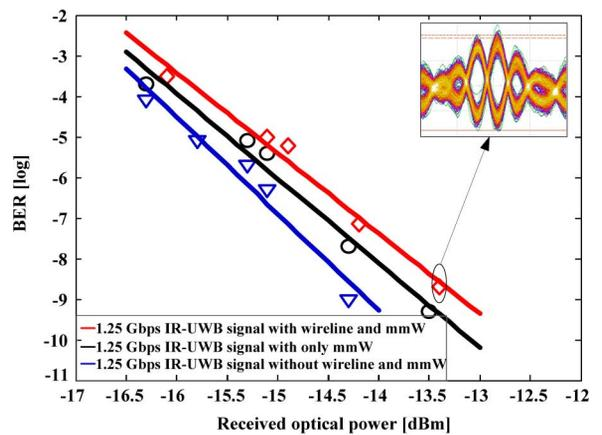
Fig. 11. BER for transmission of a 1.25-Gbps IR-UWB signal with or without simultaneous transmission of a 10-Gbps wireline signal and 1.25-Gbps 58.32-GHz mmW signal. Inset: eye-diagram of the 1.25-Gbps IR-UWB signal.
