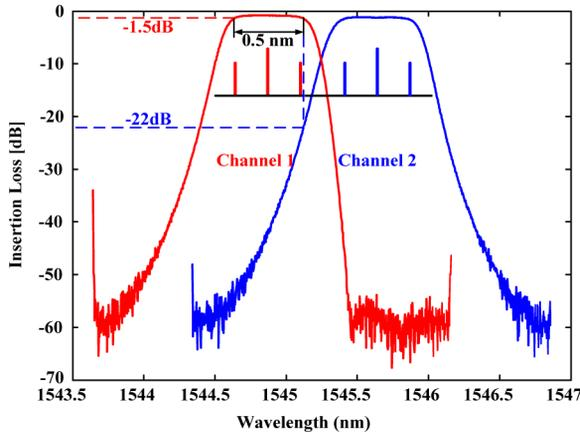
Fig. 2. Characterization of a 100-GHz spaced DWDM DEMUX and the spectral allocation for a WDM channel.
