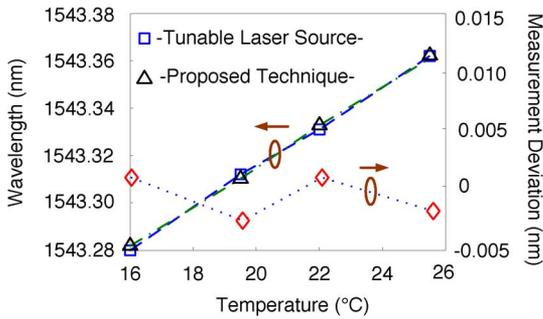
Fig. 6. Measured Bragg wavelength by the proposed technique and the use of a PD and a tunable laser source.
