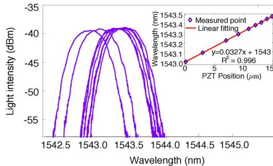
Fig. 3. Spectrum and wavelength shift of a designated AWG channel as a function of the beam position.
