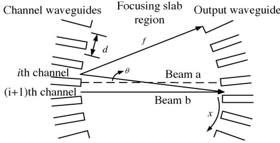
Fig. 1. Enlarged view of the second focusing slab region.
