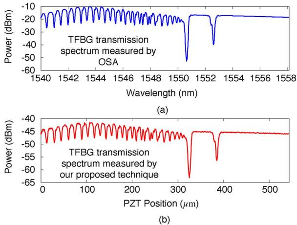
Fig. 8. Measured transmission spectrum of a TFBG. (a) Measured by an OSA. (b) Measured by the proposed interrogation technique.
