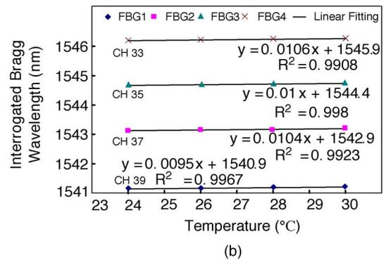
Fig. 7. Interrogation of a four-distributed-FBG sensor. (a) Shifted spectrum of each AWG channel with changed position of the input light beam. (b) Measured temperature sensitivity.
