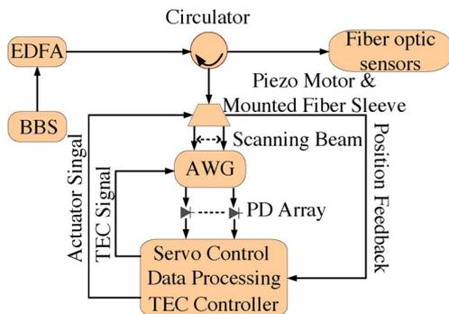
Fig. 4. Experimental setup of the proposed interrogation technique based on space-to-wavelength mapping using a closed-loop piezo motor.
