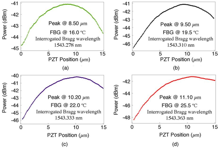
Fig. 5. Interrogation result of a single FBG sensor under four different temperatures, (a)–(d), as a function of the beam position.
