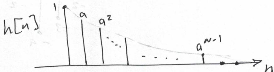
(c) Even though the system has a feedback (recursive system), its impulse response is finite. Hence, the system is FIR
