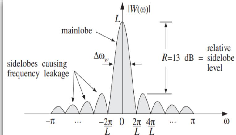
$$\Delta\omega \geq \Delta\omega_w = \frac{2\pi}{L}$$
