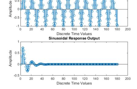
Sinusoidal 60 Hz Signal sampled at 1000 Hz sampling rate
