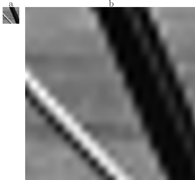
Fig. 4.5 Difficulties with the Statistical Algorithm ( 100\times Surface Magnification): a) Original LR image, b) Bayesian HR estimate
