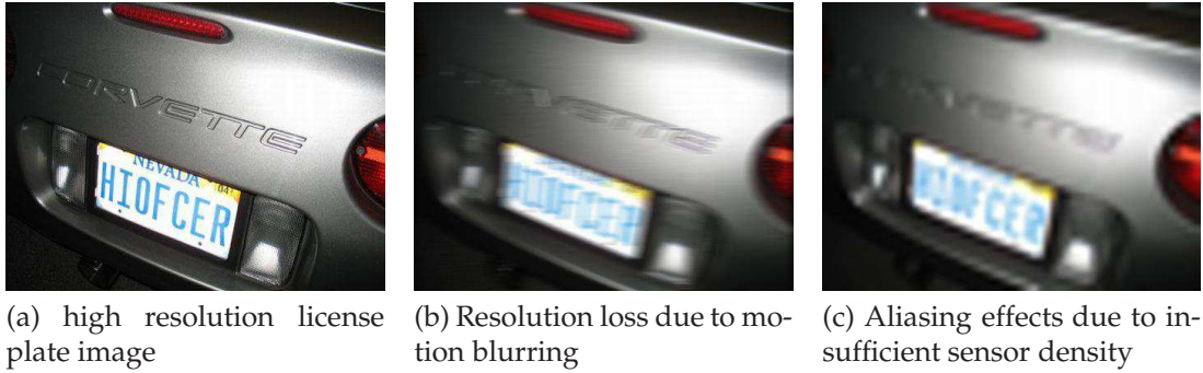
Figure 1.1: Blurring and aliasing effects in the loss of resolution
