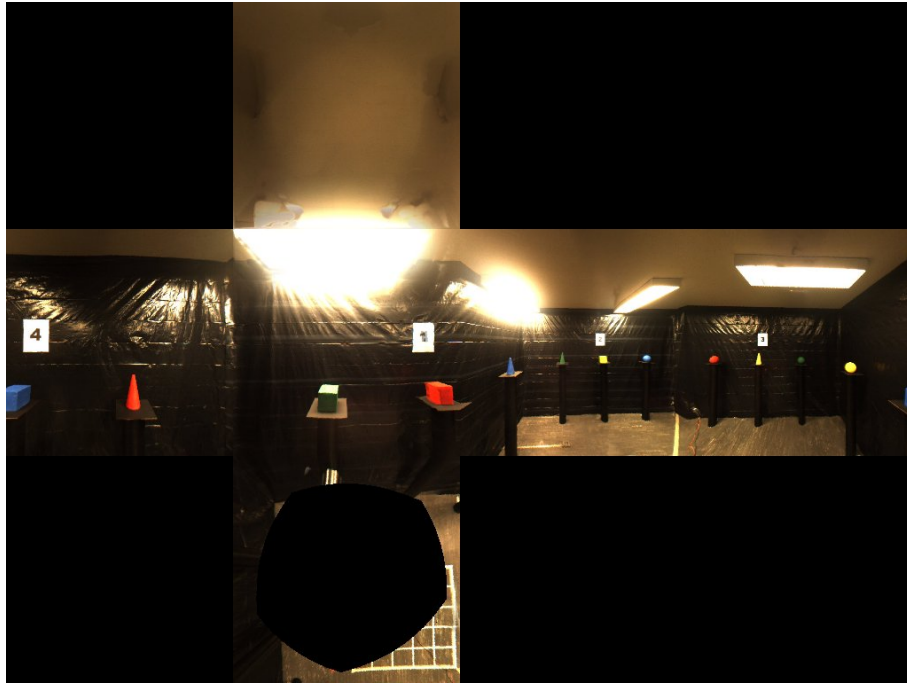
Figure 5.6: Flattened or unfolded cubic panorama of an indoor scene generated by uniform depth stereo matching.
