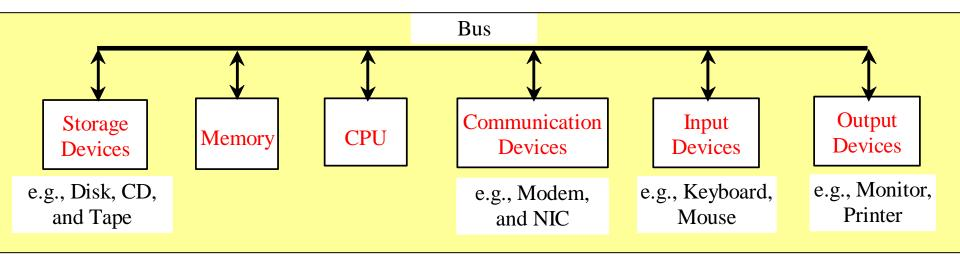
The central processing unit (CPU) is the brain of a computer. It retrieves instructions from memory and executes them. The CPU speed is measured in megahertz (MHz), with 1 megahertz equaling 1 million pulses per second. The speed of the CPU has been improved continuously. If you buy a PC now, you can get an Intel Pentium 4 Processor at 3 gigahertz (1 gigahertz is 1000 megahertz).
