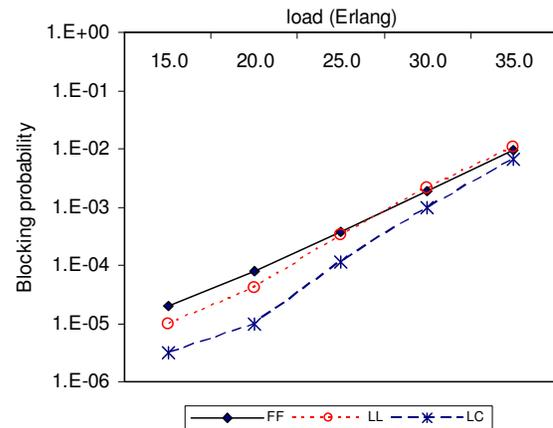
Fig. 5. Comparing LC to LL in multi-fiber networks (3 fibers per link)
