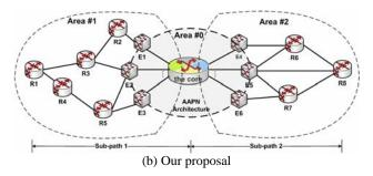
Fig. 4: The framework we proposed deploys AAPN as backbone area #0.
