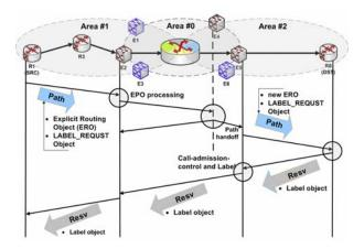
Fig. 5: Inter-area LSP signaling process
