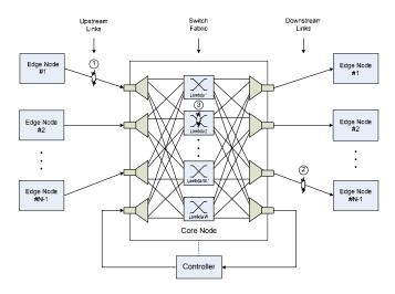
Figure 2 Illustration of failure scenarios
