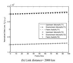
Figure 5 Data loss versus frame size
