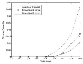
Figure 3 Blocking probability versus traffic load
