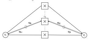
Figure 2 A set of two-hop paths between a pair of edge nodes
