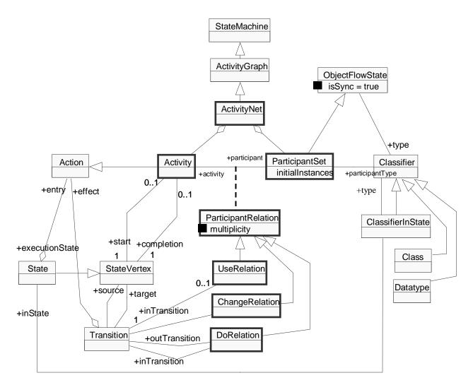
Figure 3: Abstract syntax of Activity Net concepts and their mapping to the concepts of UML Activity Graphs and State Machines
