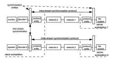
Figure 2. Example of a configuration with media synchronization.
