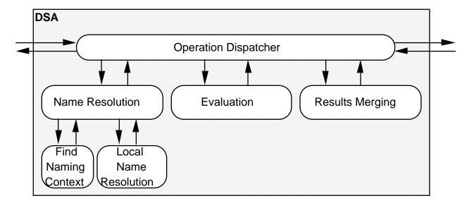
Figure 5: DSA Behavior - Internal View [X.518 88] Figure 10
