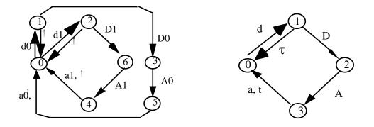
Fig.10 The modified channel specification with constraints: Chab' and Chns'.
